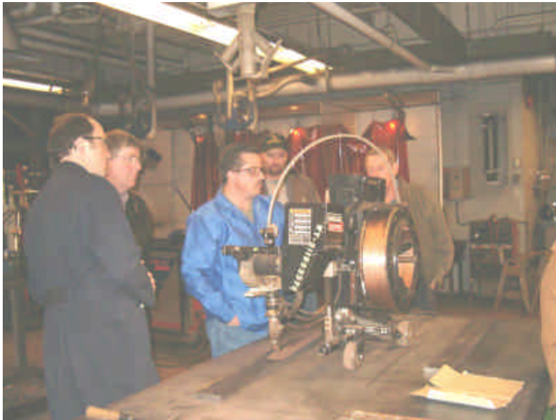
Joel Girard (far left) and Gerard Pickett (in middle) demonstrate the SAW in action.
