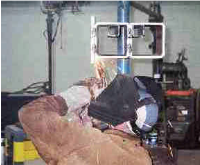
Figure 1: Overhead welding of test specimen at Walters Inc.
